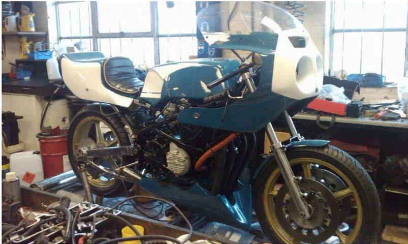
We have had to fabricate a belly pan for the event, this is due to recent regulations that require each four-stroke machine has the facility to hold the contents of the engine oil in an under tray in the event of a leak.
