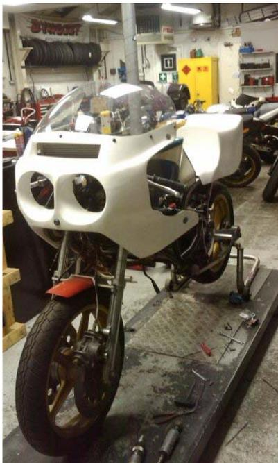
You start to get some idea of what the finished article will be like, we have two very different tanks that we might use, the square angular tank was originally designed especially for this frame and used for two seasons in Endurance races, when the bike was used for shorter distance GP races a lower more aesthetically pleasing tank was designed.
