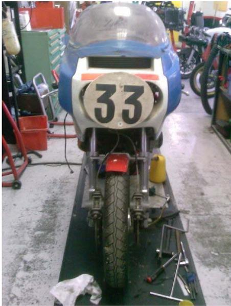
We decided to use an old fairing to make a new mold, this included the seat unit, we were able to reduce the weight of the seat unit by 2kg along...
