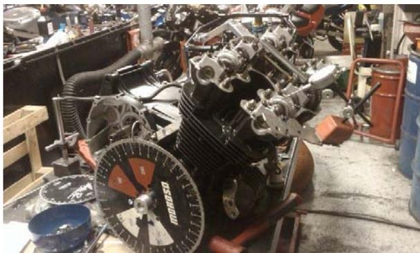
This engine, due to its uniqueness has caused us some headaches... the image on the right is one of these... The lift on the special Cams is so large that many hours were spent ensuring that we correctly 'dialed-in', we don't want to undo all the hard work and effort...!
